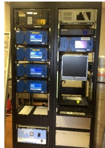
Figure 4. TEOM, NO x , SO 2 , O 3 equipment- Okanagan College
