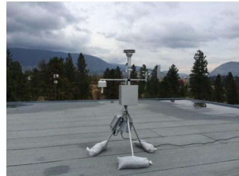
Figure 15. E-BAM installed at Johnson Bentley in West Kelowna
