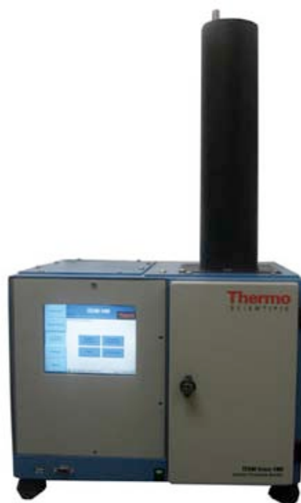
Figure 12: TEOM Monitor (ThermoScientific)
