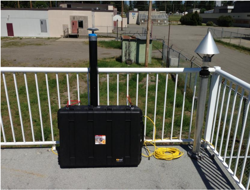
Figure 3. The fixed nephelometer in its black case, on top of the air quality monitoring station at Quesnel Secondary School.
