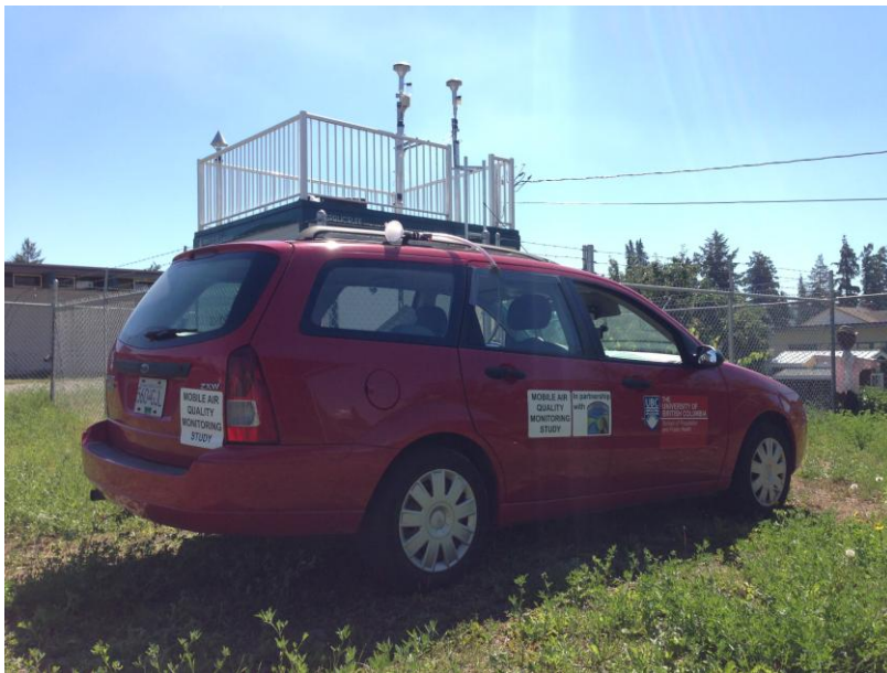
Figure 2. The mobile monitoring vehicle parked at the MOE air quality monitoring station at Quesnel Secondary School, where the fixed nephelometer was located.
