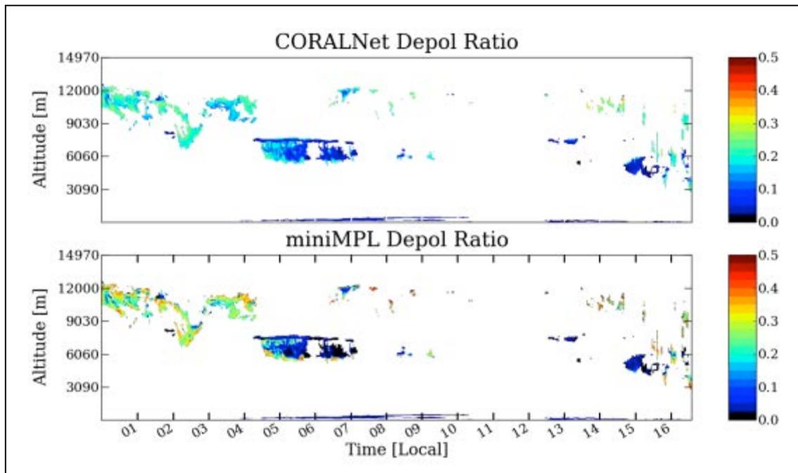
Figure 5: Masked depolarization ratio plots for CORALNet (top) and mini-MPL (bottom) from October 15, 2013. The case here is not as clear-cut in that the mini-MPL shows regions of higher
