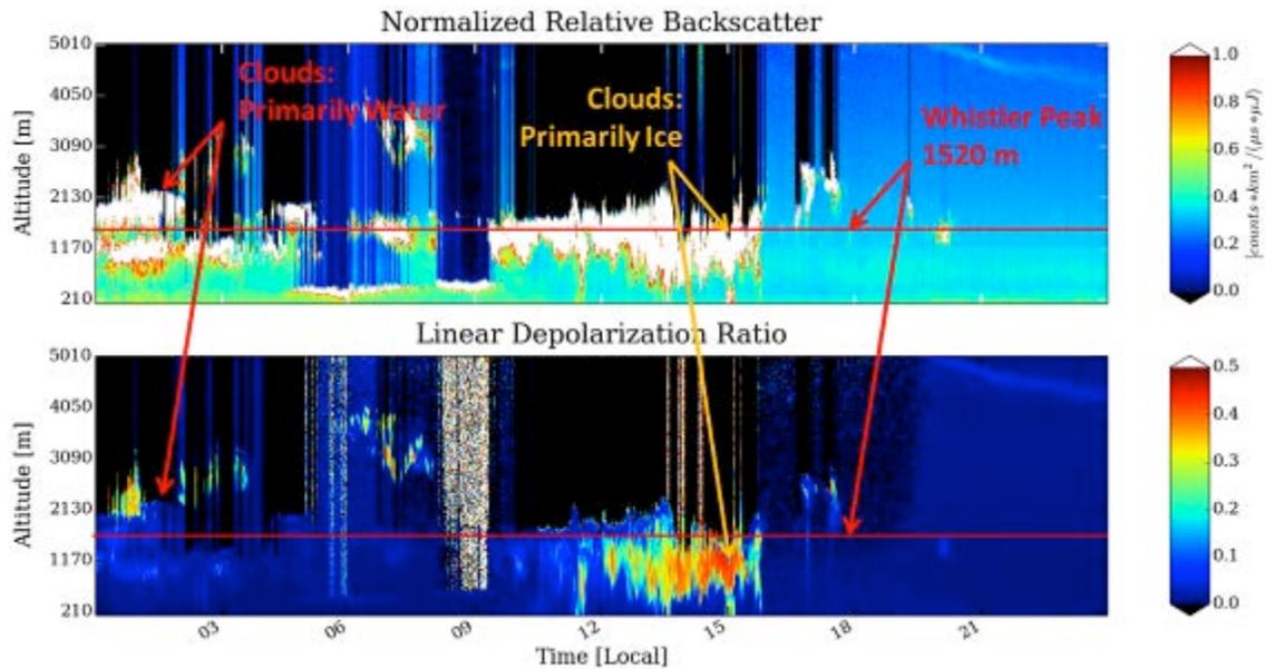
**Figure 3: Mini-MPL returns for March 20, 2014. On this day, the PBL did not extend above ~1170m AGL. Clouds near the peak consisted of mostly liquid water until ~12:00, when icier clouds emerged.**
