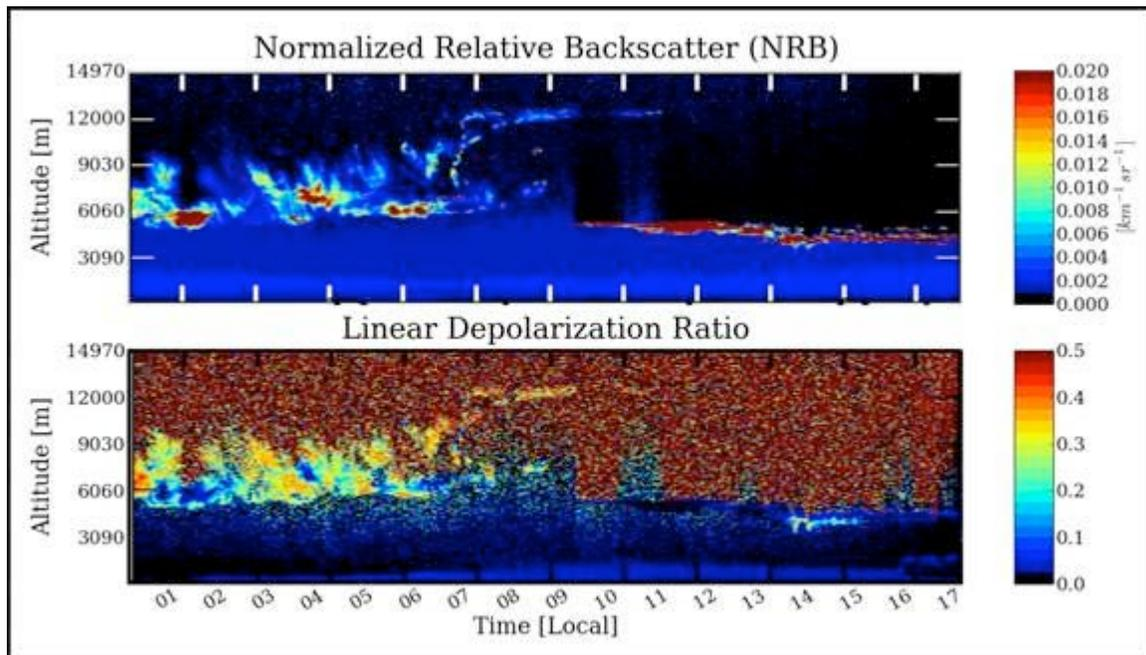
**Figure 2: False colour plots of normalized relative backscatter (top) and linear depolarization ratio (bottom) taken by the mini-MPL on September 19, 2013. Cirrus clouds can be seen from 6,000-12,000 m during the first half of the day. These clouds show depolarization ratios from <0.1 up to 0.5.**
