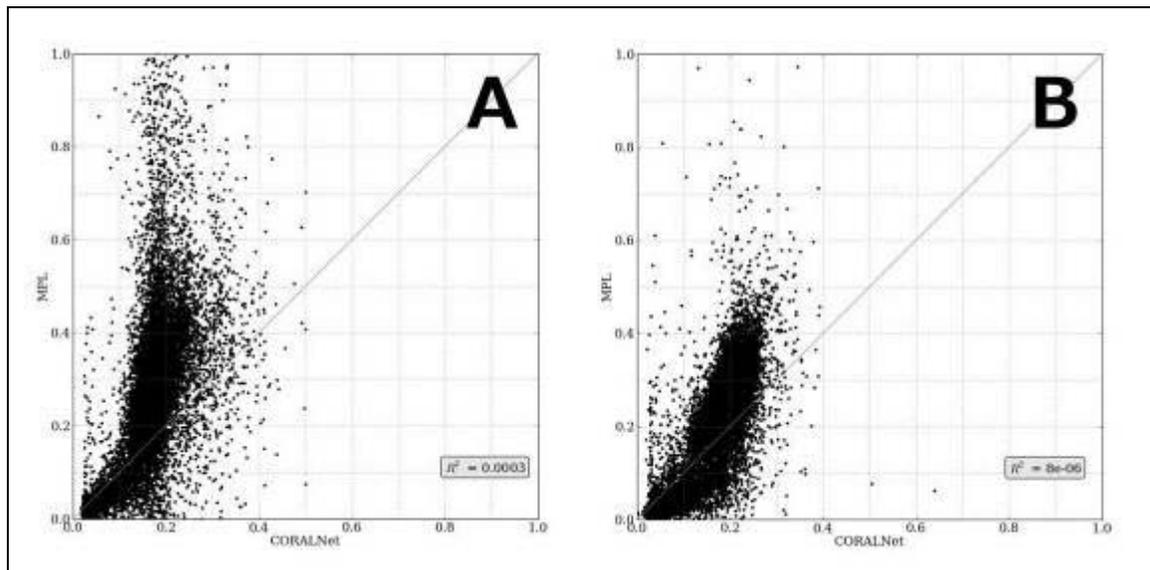
**Figure 8: Scatterplots comparing depolarization results for CORALNet and mini-MPL. Plot A shows results for September 19, 2013 and Plot B shows results for October 15, 2013. In both plots, the relationship is consistent and clear: the mini-MPL shows higher depolarization ratios than the CORALnet lidar. However, the relationship is not necessarily linear.**
