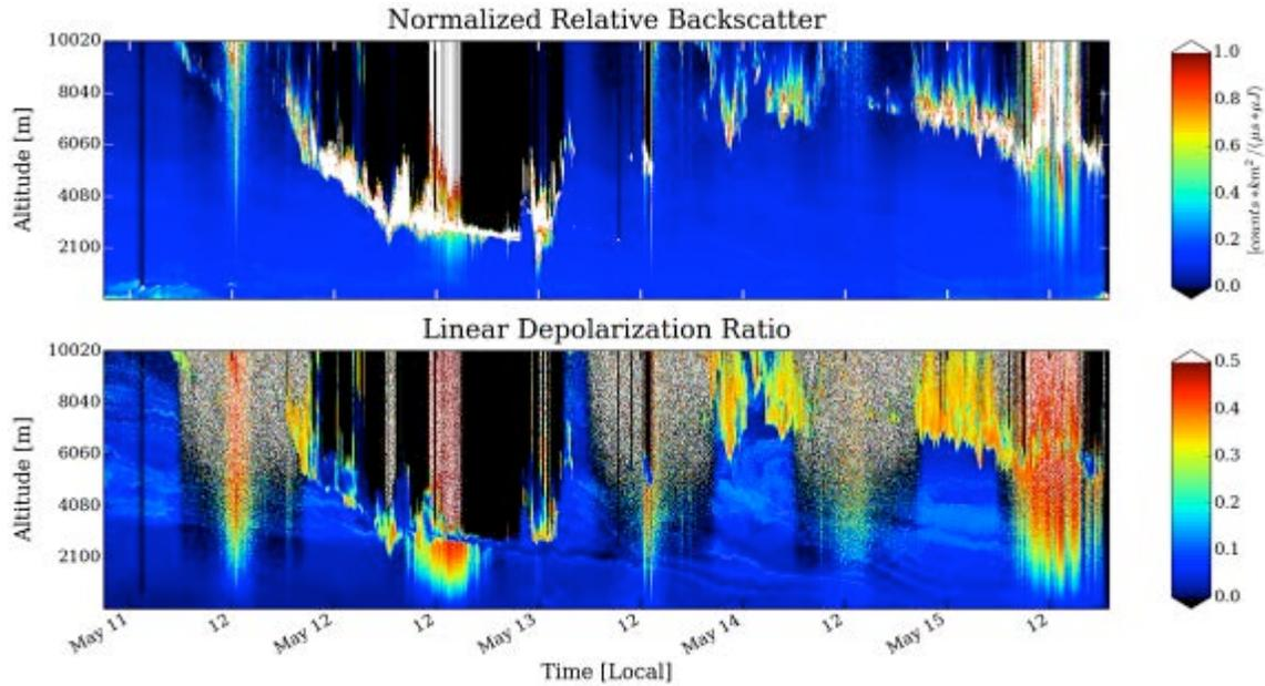
**Figure 11: Lidar returns from May 10-15, 2014. Multiple layers of aerosols observed from 2-10km with depolarization ratios varying from 0.12-0.22. As in the results from May 05-08, these layers have been associated with outflows of aerosols from Asia.**
