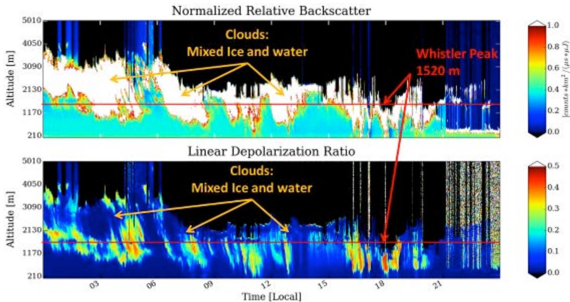
**Figure 4: Mini-MPL returns for March 27, 2014. On the 27<sup>th</sup>, the peak passed into and out of ice and water clouds intermittently throughout the day. In between, it appears that periods of elevated aerosols levels were seen at the peak.**
