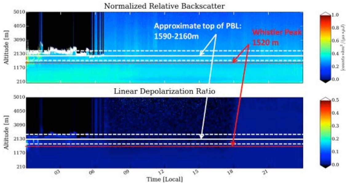
**Figure 2: Mini-MPL data from Feb. 28, 2014 showing Whistler peak within the PBL. Altitudes are measured in AGL units from the valley floor, putting the peak at 1520m.**
