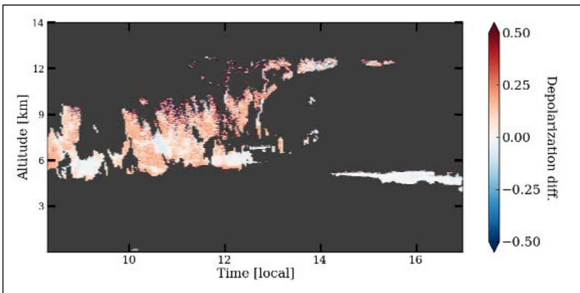
**Figure 6:** Plot of the difference in polarization results between the two systems for September 19, 2013. In this plot, positive values indicate the mini-MPL depolarization was higher than that from CORALNet.
