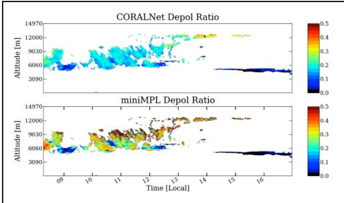
Figure 4: Masked depolarization ratio plots for CORALNet (top) and mini-MPL (bottom) for September 19, 2013. A quick comparison of the two shows the CORALNet ratios appear to be markedly lower than those measured by the mini-MPL. In this plot, only the strongest signal levels are left unmasked to reduce the effects of noise.
