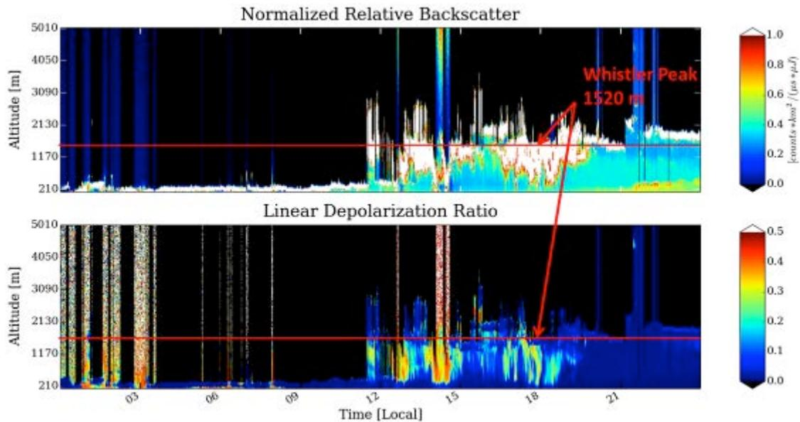
**Figure 5: Mini-MPL returns for March 30, 2014. No useful observations before 12:00 due to low clouds. After that, the peak sees intermittent clouds and aerosol layers.**
