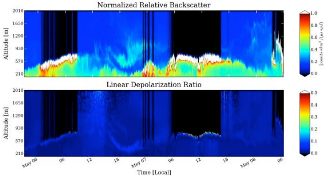
**Figure 10: Lidar returns focusing on the planetary boundary layer over Amphitrite Point from May05-08, 2014. This diurnal effect is typical of the daily encroachment of a marine layer.**
