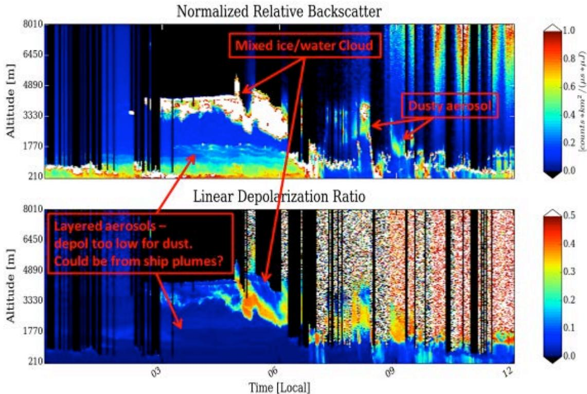
**Figure 8: Lidar returns from the morning of May 03, 2014. This day is a good example of the complexities that can be observed at this location. The early hours of the morning was typified by a deep boundary layer, topped with intricate layers of highly spherical aerosols up to ~2000m. Then, from 7:00AM to noon, light rain cleared out the aerosols near the surface while dusty aerosols interacted with thin clouds from 1500-3000m.**
