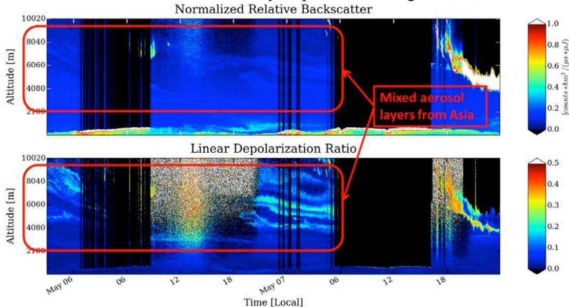
**Figure 9: Lidar returns from May 05 - May 07, 2014. During this period, aerosol returns from 2-10km were connected to strong outflows of dust and smoke from Asia.**
