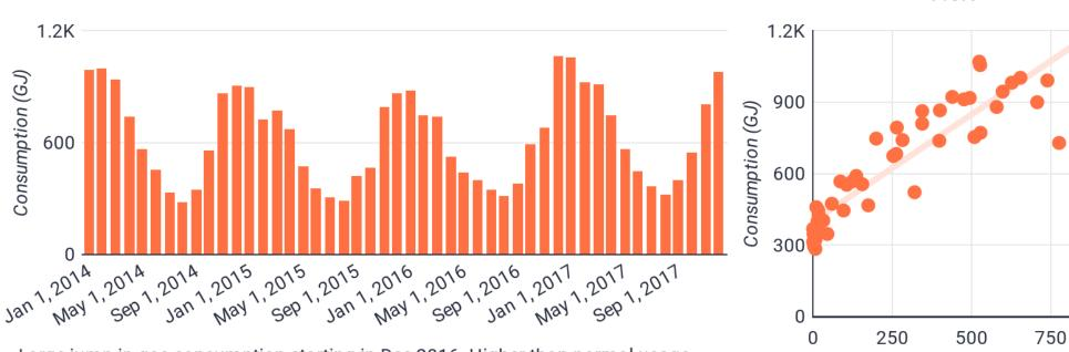
Large jump in gas consumption starting in Dec 2016. Higher than normal usage appears to continue to present, should be investigated. Possible causes include longer run hours or increased outside air intake. Overall consumption is high compared to average values.
