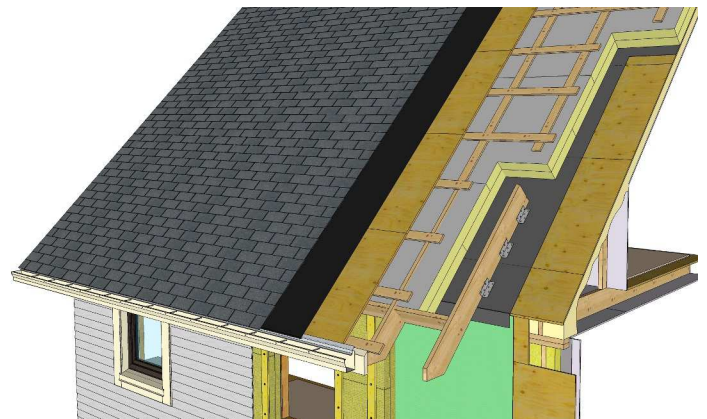
Interior and exterior insulating strategies as part of retrofitting procedures for the whole house.
