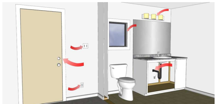
Above-grade wall air sealing locations discussed in the guide.
