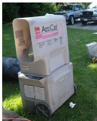
Blown-in insulation prior to installation and blowing machine.
