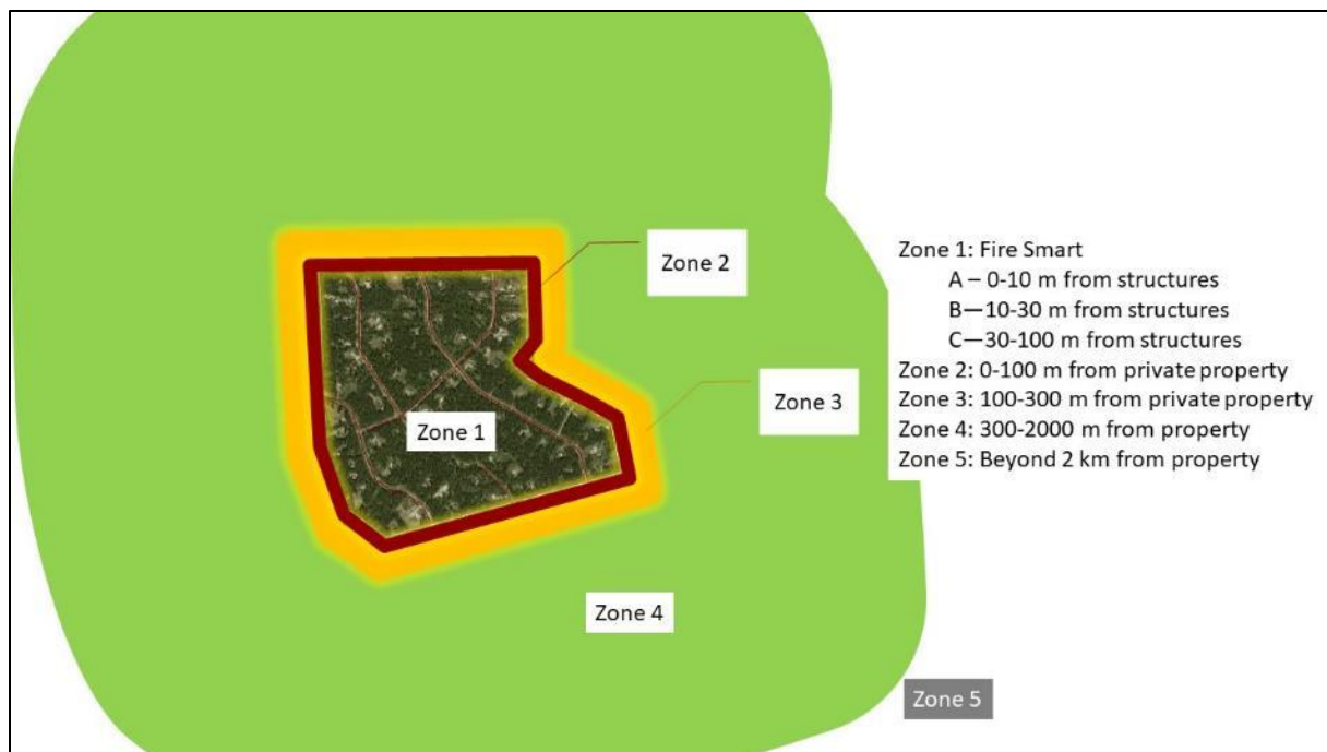
Figure 4: Five zones based upon distance from structures inform both treatment priority and the nature of treatments.
