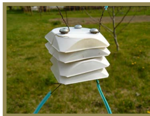
iButton temperature data logger weather shield
