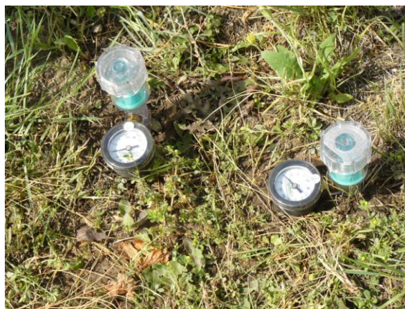
Tensiometers installed at 30 and 60 cm at all test vineyards
