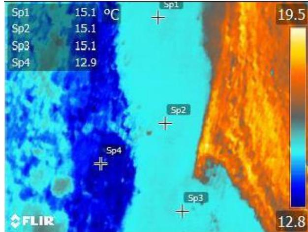
In addition to the individual FLIR images of potential groundwater inputs, a stitched thermal map layer of the stream sections that were flown was created using Pix4D Mapper Pro (Educational Version). The imagery was processed in small batches (typically 10 to 50 images) in order to optimize the image stitching procedure. Stitched images were exported in TIFF format and were added to the GIS map, noted previously (Figure 2).
