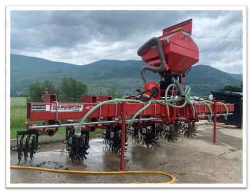
Figure 18 - Lilliston cultivator with Einbock pneumatic seed box
