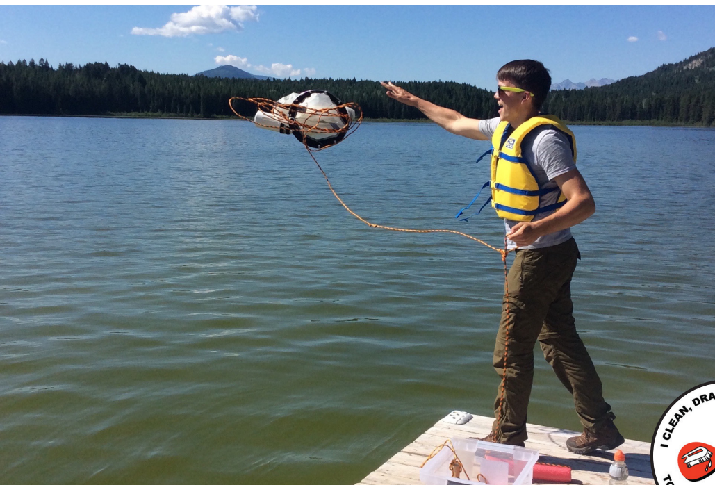
Here, a CSISS staff person deploys monitoring equipment to check for zebra and quagga mussel larvae, which are tiny and free swimming. To date, zebra and quagga mussels—adult or larvae—have not been detected in the Shuswap watershed. Photo credit: Columbia Shuswap Invasive Species Society
