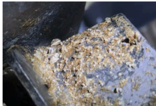
Invasive mussels found on the trim tabs of a cabin cruiser from Michigan. The Surrey inspection crew completed a full decontamination of the watercraft.
