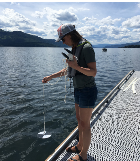
Staff prepare to lower a Secchi disk to take a water quality reading. The Secchi disk gives an indication of water clarity.
