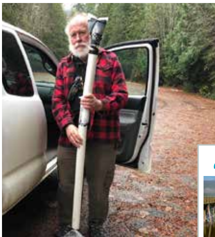
A member of the research team holds the 2-metre sediment core collected from the bottom of Mara Lake.
