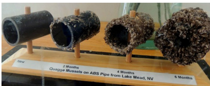
This photo shows how quickly quagga mussels have colonized on pieces of pipe in Lake Mead (Nevada) over different periods of time. This imposes very costly ongoing maintenance to rid pipes and other infrastructure of mussel colonies.
